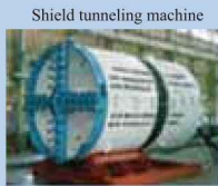
Shield tunneling machine
